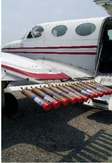
Operasi Pembenihan Awan dengan kaedah hygroscopic flare Cloud seeding operations using the hygroscopic flare method
